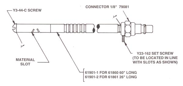
✓ USE PERM-LOK SEALANT ON THREADS
